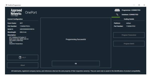
Confirm successful programming by verifying that the Part Number on the left-hand side matches with the part number chosen and noted down prior to programming.
