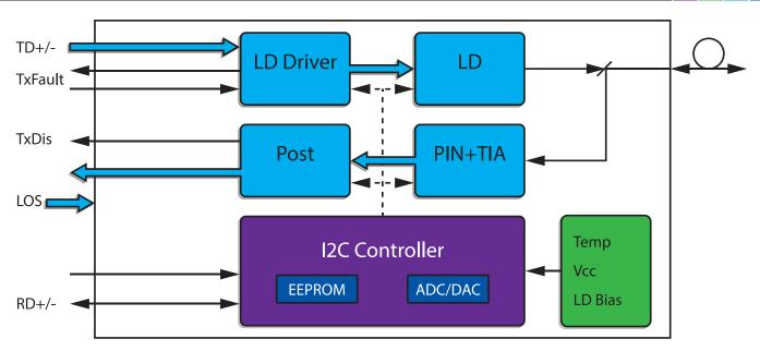
Figure 1. Transceiver functional diagram
